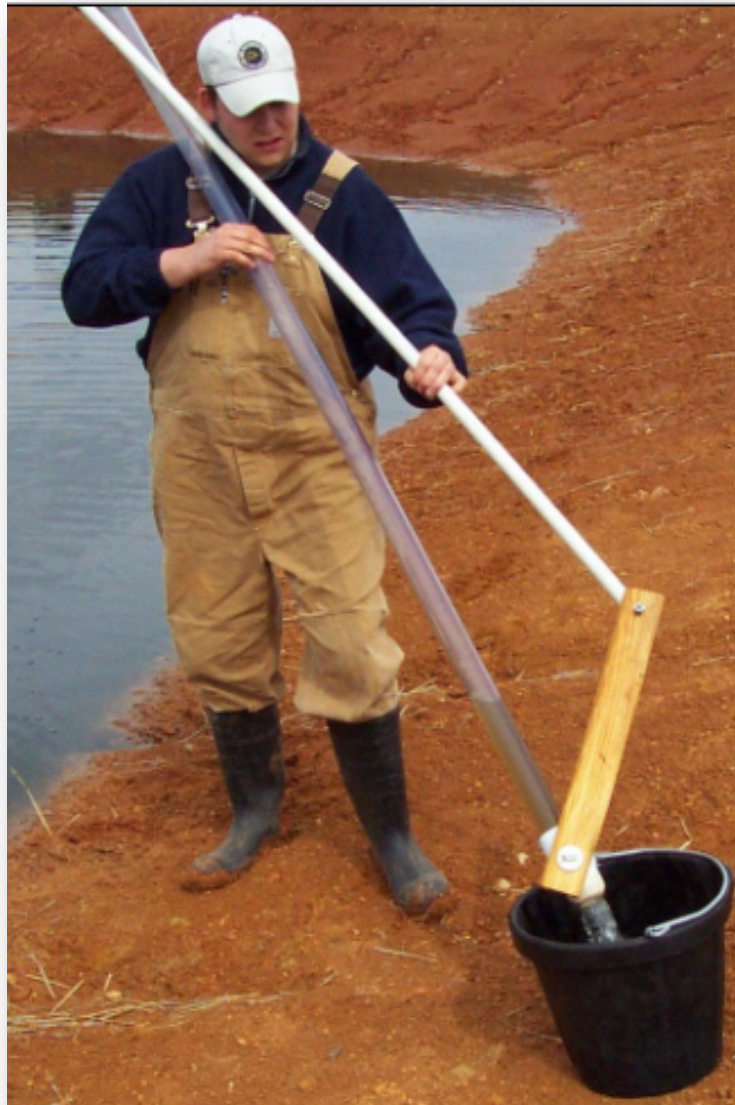
Photo 4. Foot valve manure sampler as used to collect samples from the C&H lagoon.
