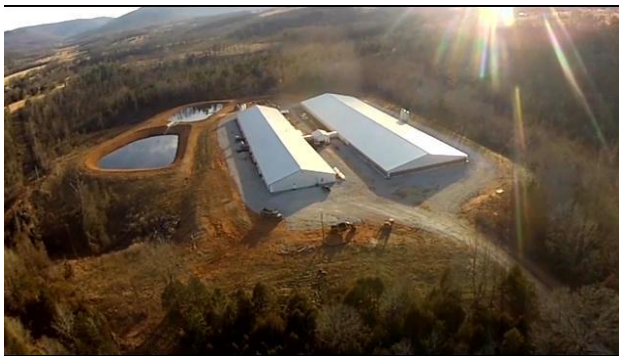
Figure 2. Areal view of 6,500-head industrial hog CAFO, including waste lagoons. The facility is sited on the Boone Formation, a karst aquifer less than 10 kilometers upstream from the confluence of Big Creek with the Buffalo National River.
