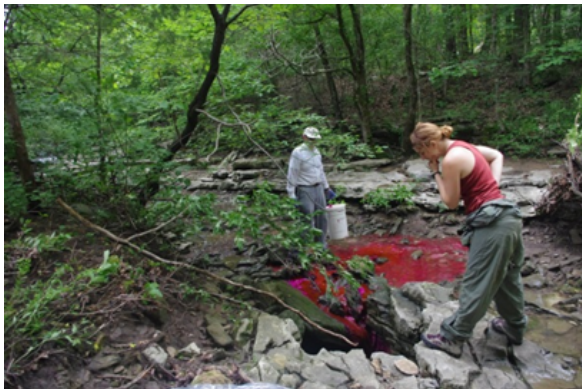
Figure 6. Swallet in Dry Creek in Ozark National Forest capturing all streamflow upgradient from CAFO spreading fields. In karst, surface water and groundwater interact as a single resource, with streams typically being pirated into groundwater as shown here, later resurging from downgradient groundwater springs back to the surface.
