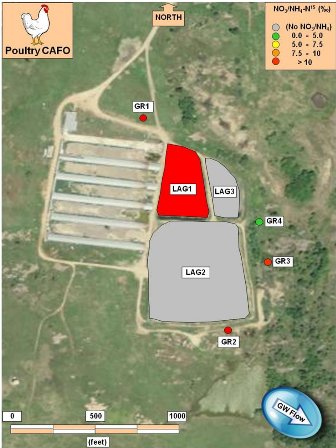
Figure 3. CAFO Site #2 schematic (poultry layer operation, since closed). Colors of decommissioned lagoons and wells correspond to ranges of \delta^{15}\text{N} of nitrate or ammonium as shown in legend at upper right, based on 2009 data.
