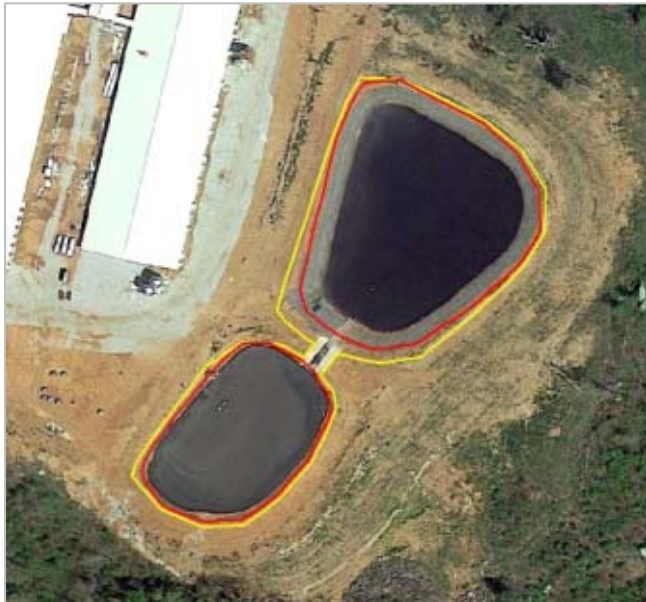
Figure 4. More magnified view of the large swine waste “manure” or “slurry” holding ponds as described by the BCRET. The yellow outer boundary was described as denoting the drainage area (59,457 square feet) into the waste holding ponds. The red inner boundary was described as denoting the top of the free board for holding pond 1 (16,999 square feet) and the larger holding pond, holding pond 2 (34,618 square feet). The volumes of waste holding ponds 1 and 2 were given as 616,395 gallons and 1,723,009 gallons. From the BCRET quarterly progress report dated October 1 to December 31, 2014, pp. 35-36.
