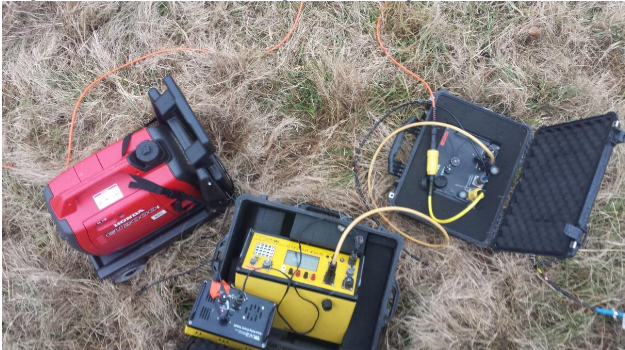
Figure 1 – ERI equipment set up (Power Supply – AGI SuperSting R8/IP Resistivity Instrument - Switch Box - Electrode cables).
