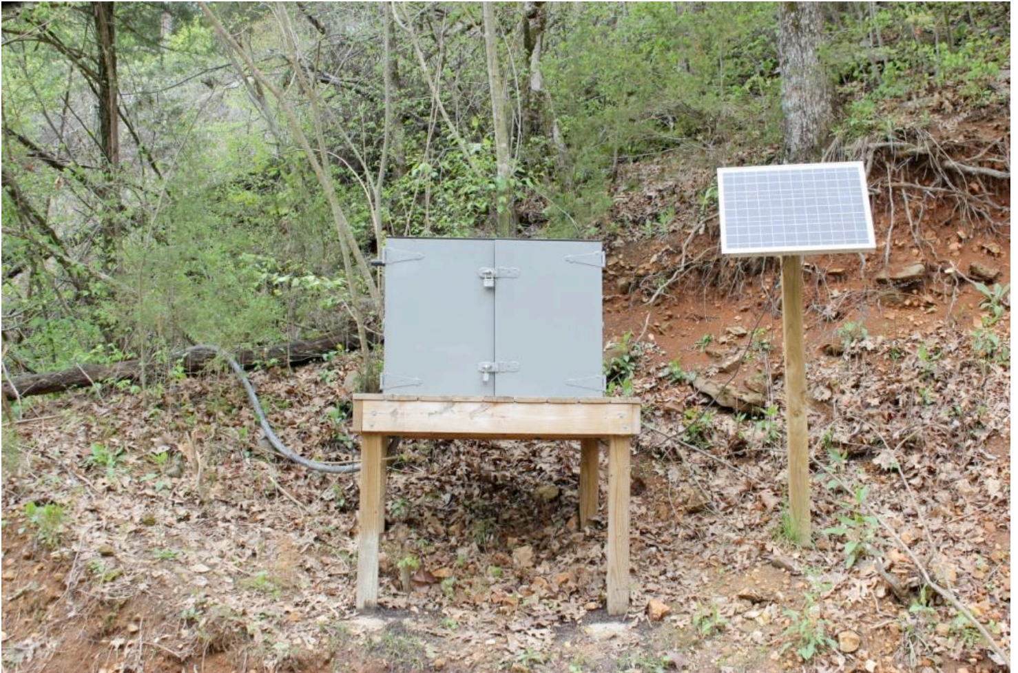
Automatic Water Sampler Upper End of the main fork of Big Creek.
