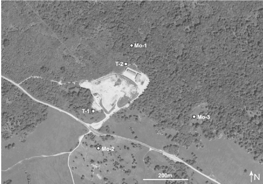
Fig. 3 The landfill with the two injection points (T-1, T-2) and the monitoring boreholes (Mo-1, Mo-2, Mo-3) (Topographic base: [54])
