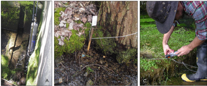
Fig. 3 Example of loggers used in recent monitoring. (a) Multiport logger with pH, conductivity, temperature, and water level sensors. (b) Temperature logger attached to a stake. (c) Data download
