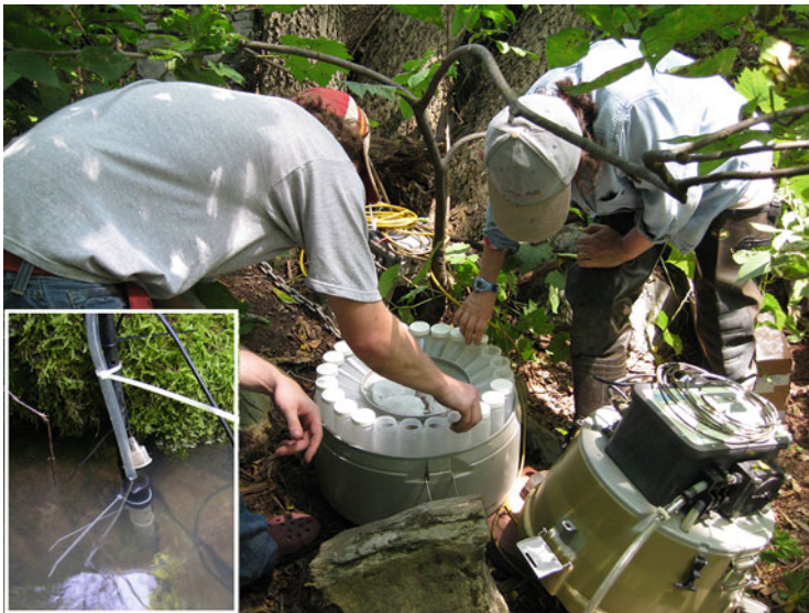
Fig. 4 Automatic ISCO stormwater sampler with 24 1-L bottles used to collected stormwater discharge at the springs. Inset shows water level trigger and pump tubing intake
