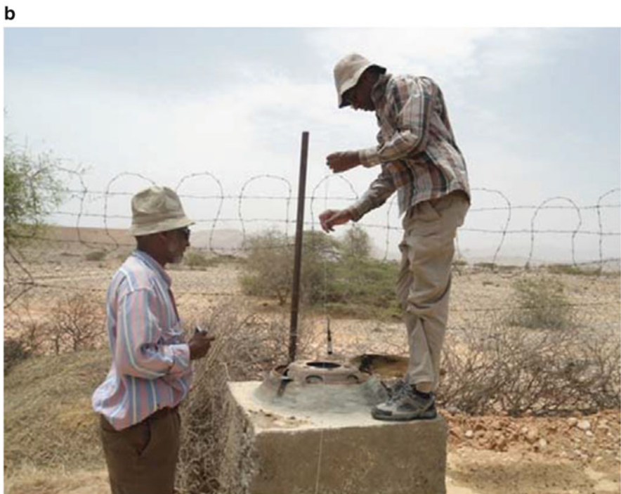
Fig. 23 Groundwater monitoring in Somaliland and Puntland: (a) map of groundwater quality of the Karkar karstic aquifer (with prevailing moderate to low quality water), (b) diver installation in Bossaso (Puntland) [51]
