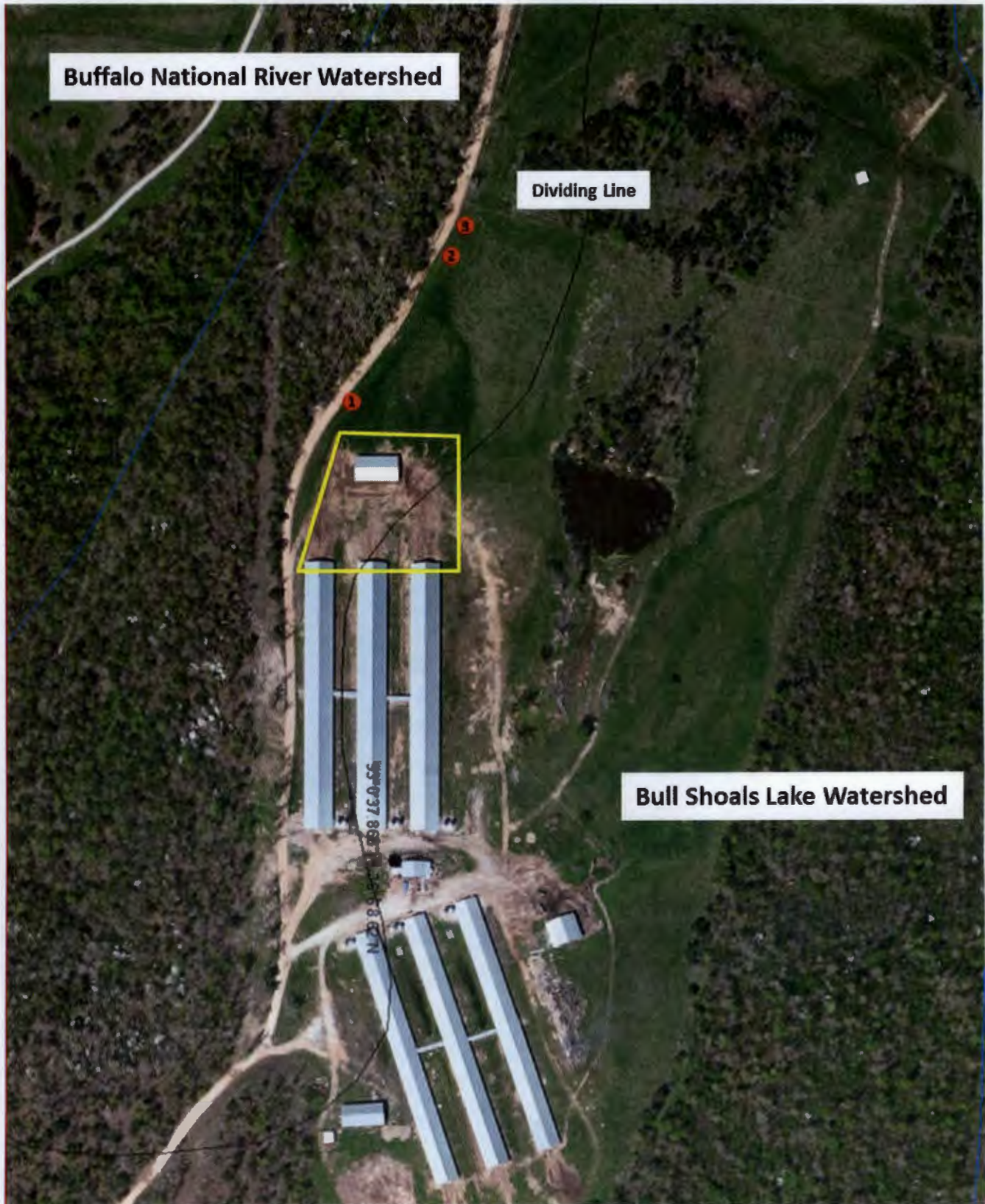
Figure 5: Map showing approximate runoff locations (red dots 1-3) from Photos #4 - #9 onto County Road 50. Area inside of the yellow box outlines pig and animal waste locations in Photos #2 & #10. All runoff observed was flowing towards Cedar Creek (blue line) in the Buffalo National River Watershed.
